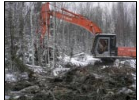
Excavator with hydraulic thumb pulling out material on Flat Creek Fire
